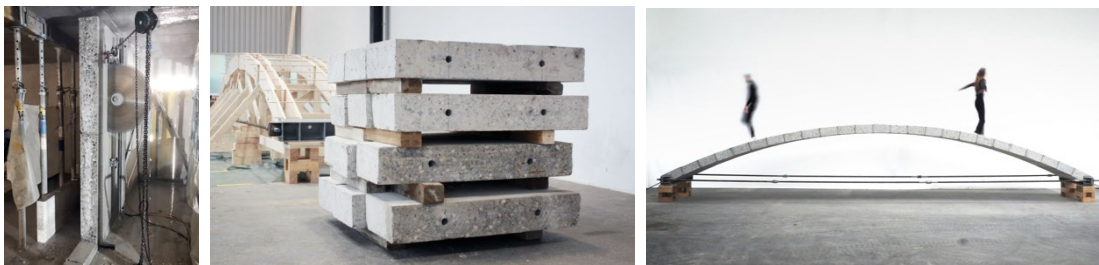
Figure 7. Footbridge built from reused concrete blocks by the Structural Xploration Lab (EPFL)
