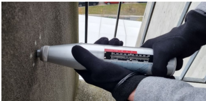
Figure 8. Schmidt rebound hammer measurements.
